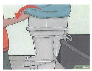
Place the cowling back onto its fittings. Clean it off, and then cover the whole motor in a canvas or plastic covering for the duration of storage.
