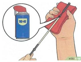
Wipe down and spray all accessible mechanical components and moving parts with an anticorrosive. Some of the best options are lubricants such as WD-40 or Quick-lube. Be sure to lubricate or grease all the moving parts such as the pivots, shift mechanism, throttle cables, carburetor valves, etc.
