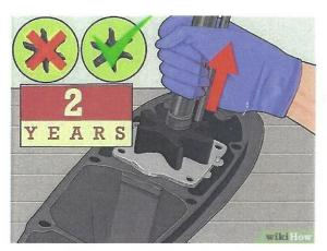
Replace the water pump impeller every two years (annually if it is used in saltwater). The impeller is a component of the pump, and it circulates water and prevents the engine from overheating. However, these tend to become jammed with muck over time, and should be replaced regularly. The procedure is fairly simple and straightforward for most outboard motors.[9]
