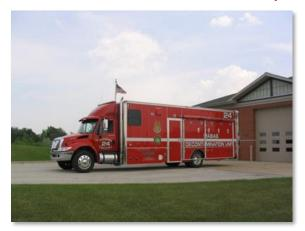
Mass decontamination – up to 200 people with supplies on board. Shower and hygiene facilities. Exterior, under-awning, misting nozzles for cooling or mass decontamination.
