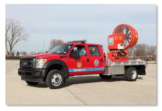
100 hp fan motor on elevating, rotating, and tilting stalk. Used for hi-rise ventilation, confined space ventilation, mass decontamination/cooling (with attachment for hose), toxic gas dissolution, etc.
