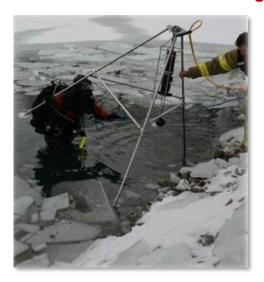
The sector scan HD sonar head is deployed to the bottom on a tripod. The system is operated from a laptop computer and high-resolution images are produced as the unit scans in a 360° view. Scanning results allow real time conditions that provide diver coordination and maximizes diver safety in order to fulfill rescue and recovery operations.
