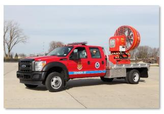
100 hp fan motor on elevating, rotating, and tilting stalk. Used for hi-rise ventilation, confined space ventilation, mass decontamination/cooling (with attachment for hose), toxic gas dissolution, etc.
